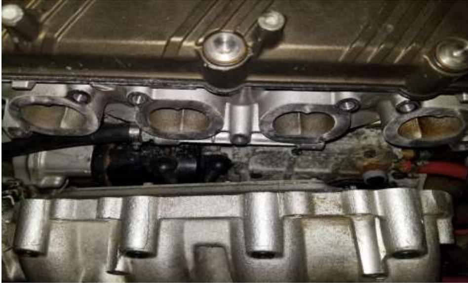
29. Remove remainder of studs. Make sure the face of the exhaust ports are clean of all gasket material and oil. You may need to block off all ports with paper towels and use the razor blade to scrape. Scotch brite may be needed also, this must be bare aluminum to seal properly. Blow with air and wipe with brake cleaner to remove oil when done.
