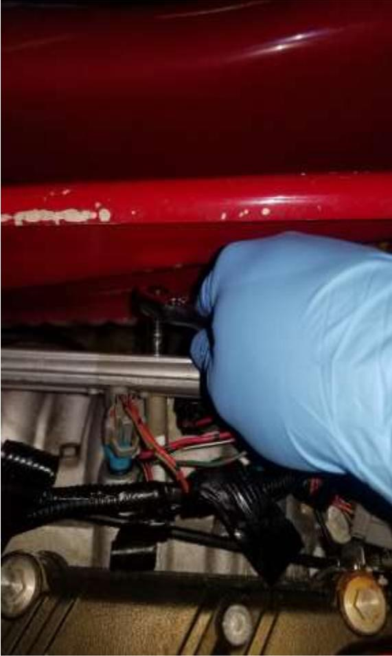
5. Remove the fuel rail using a 8 mm socket.
