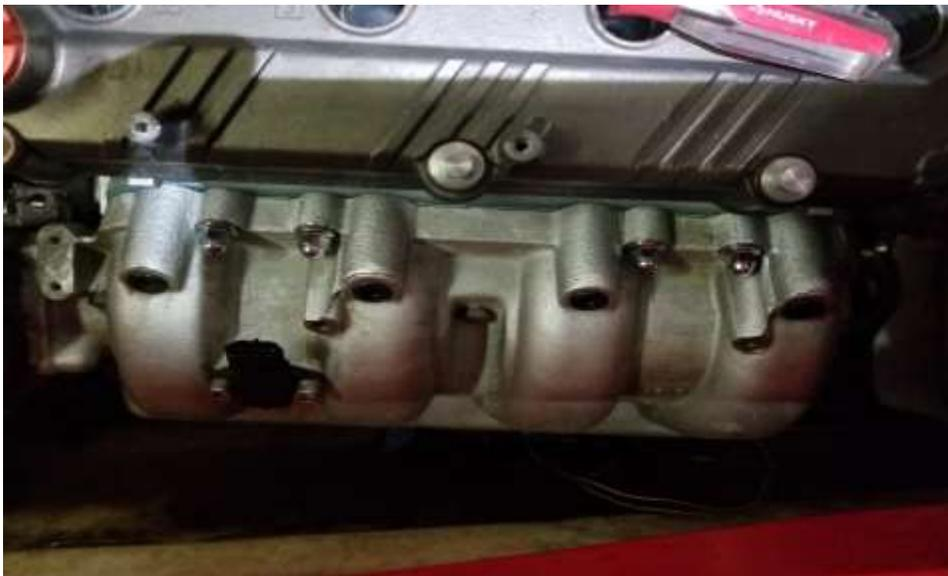
36. Place your washers and acorn nuts on the four studs, and 3 short bolts with washers as well. Tighten acorn nuts to 14 ft.lb and bolts to 18 ft.lb.
