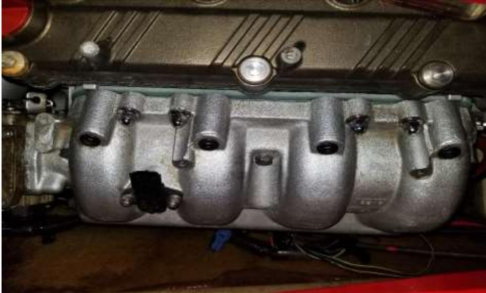
37. Your thermal barrier is installed! Now we can Assemble.
