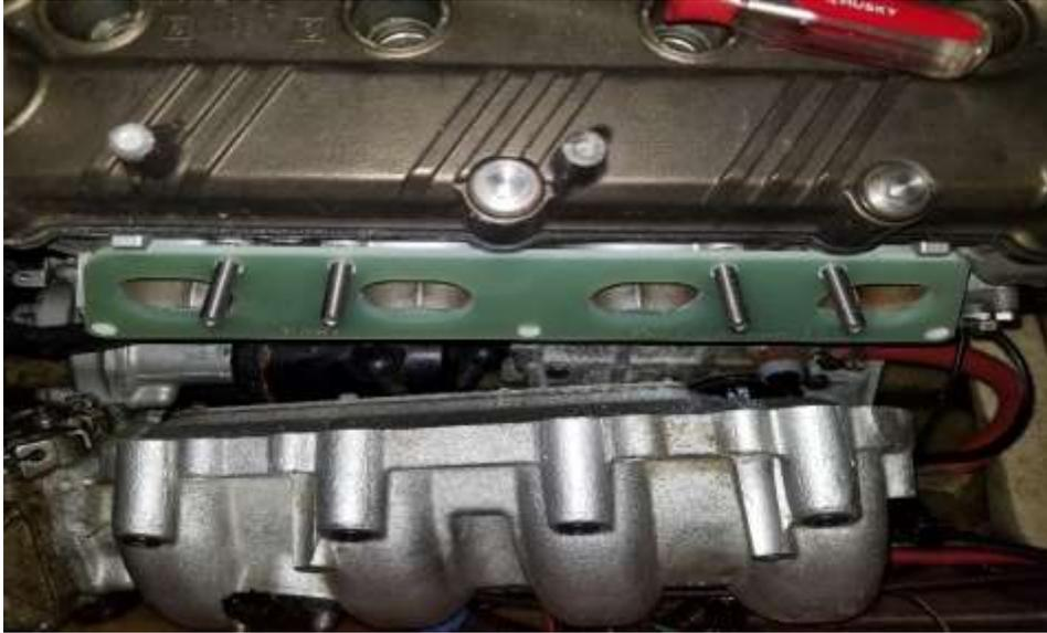
33. After the gasket has been placed on, place the thermal barrier on. Make sure the Kawi Performance logo faces you as shown.
