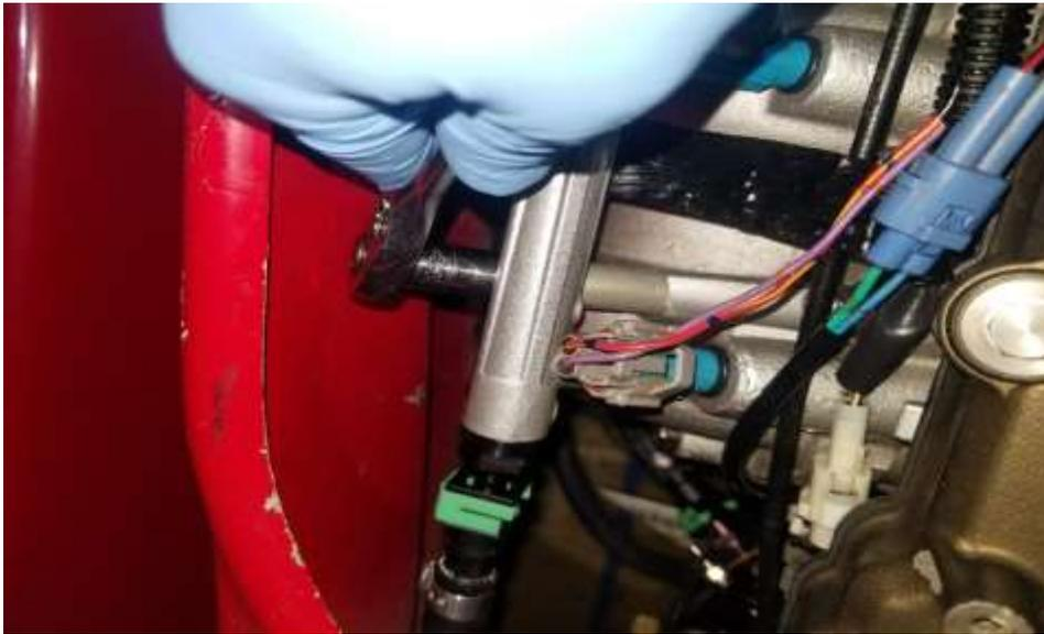
7. Continue removing each bolt using the 8 mm socket, until all are removed. Set aside.
