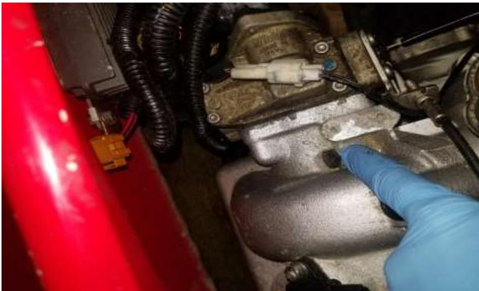
18. Locate the end bolt on the intake manifold.
