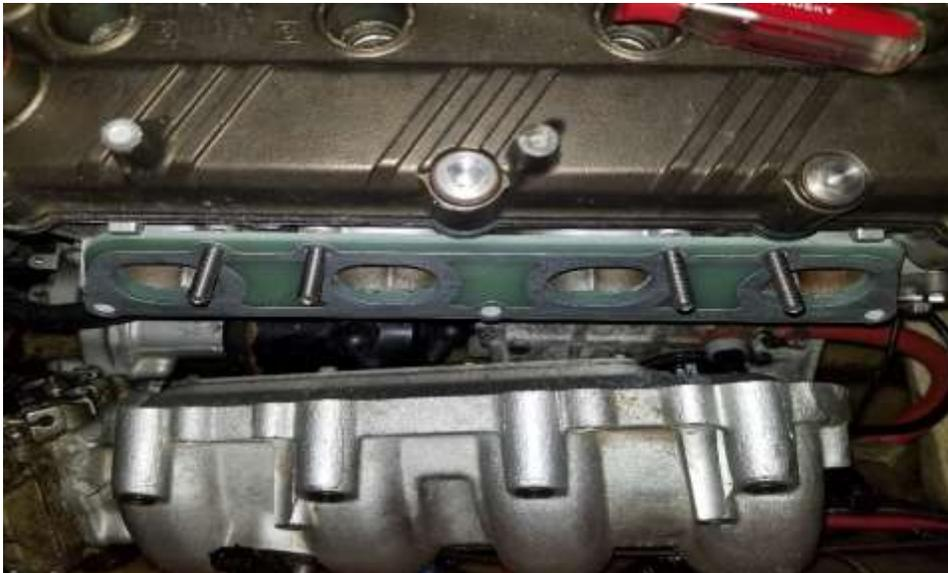
34. Place the second gasket on top of the barrier, again gasket side does not matter.
