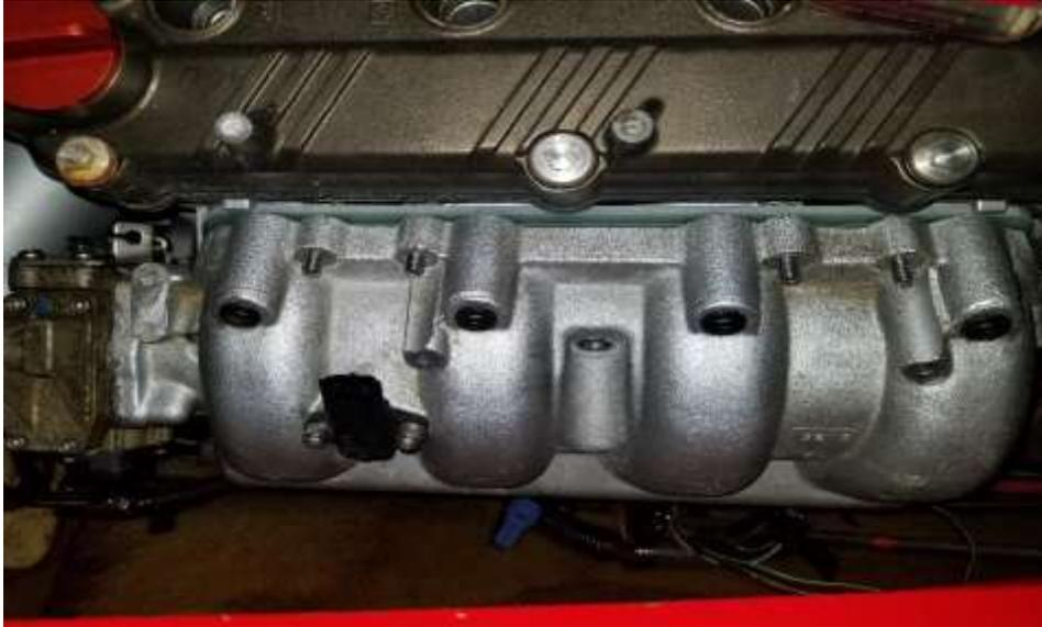
35. You can now place the manifold back onto the engine, please keep in mind the manifold must be super clean and bare aluminum as well. You may need to remove it from the hull to clean properly. You should see the four studs sticking out at the top as shown.
