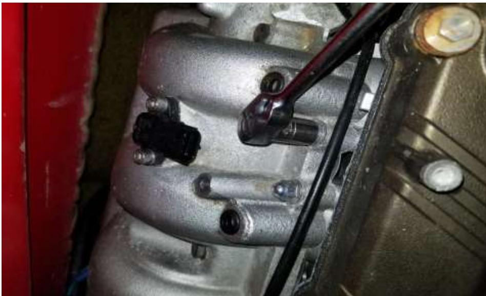
20. Remove the acorn nuts on the intake manifold using an 12mm socket.
