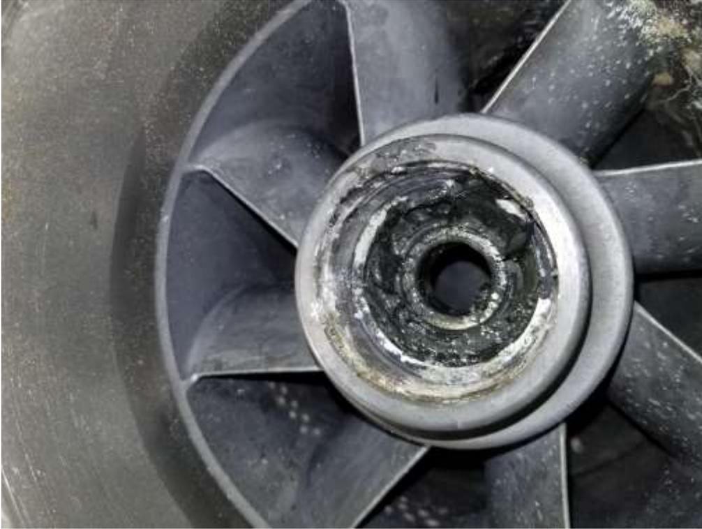
6) Take old shaft and insert it upside down as shown below. Push bearing out.
