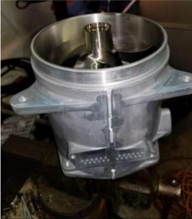
25) Insert spline tool and tighten to 110 ft.lb.
