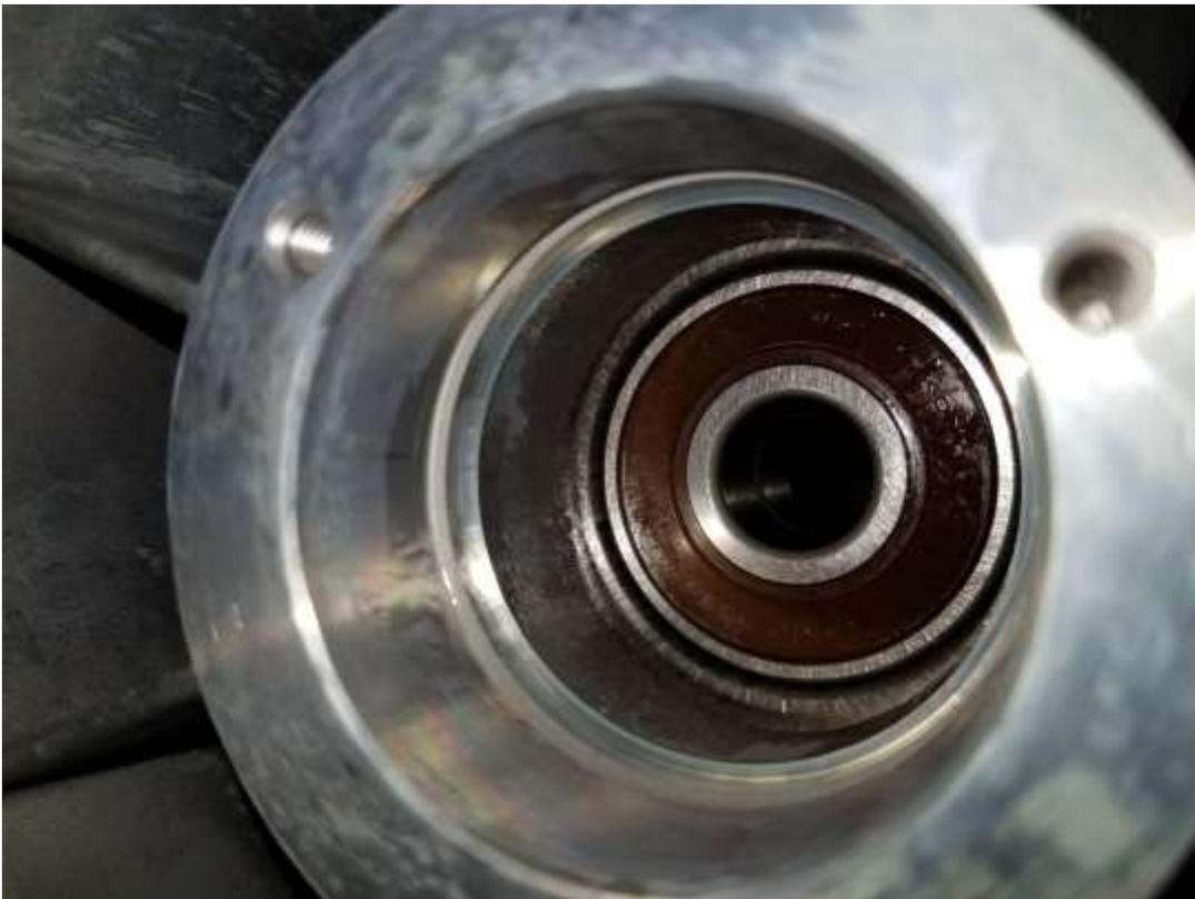
15) Flip pump over and install bushing as shown below.
