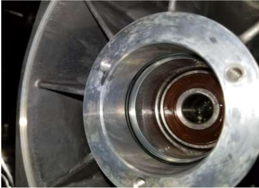
20) Install pump housing o-ring (for 300/310 Ultra LX Models only)
