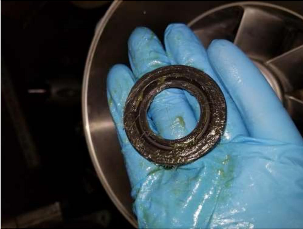
18) Pack grease on top of next seal, and repeat. Be careful not to damage the seal.
