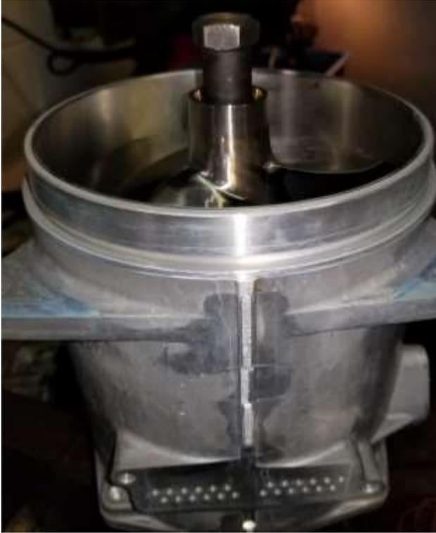
26) Remove pump and tighten spline tool in vice. Reinstall pump as shown below.
