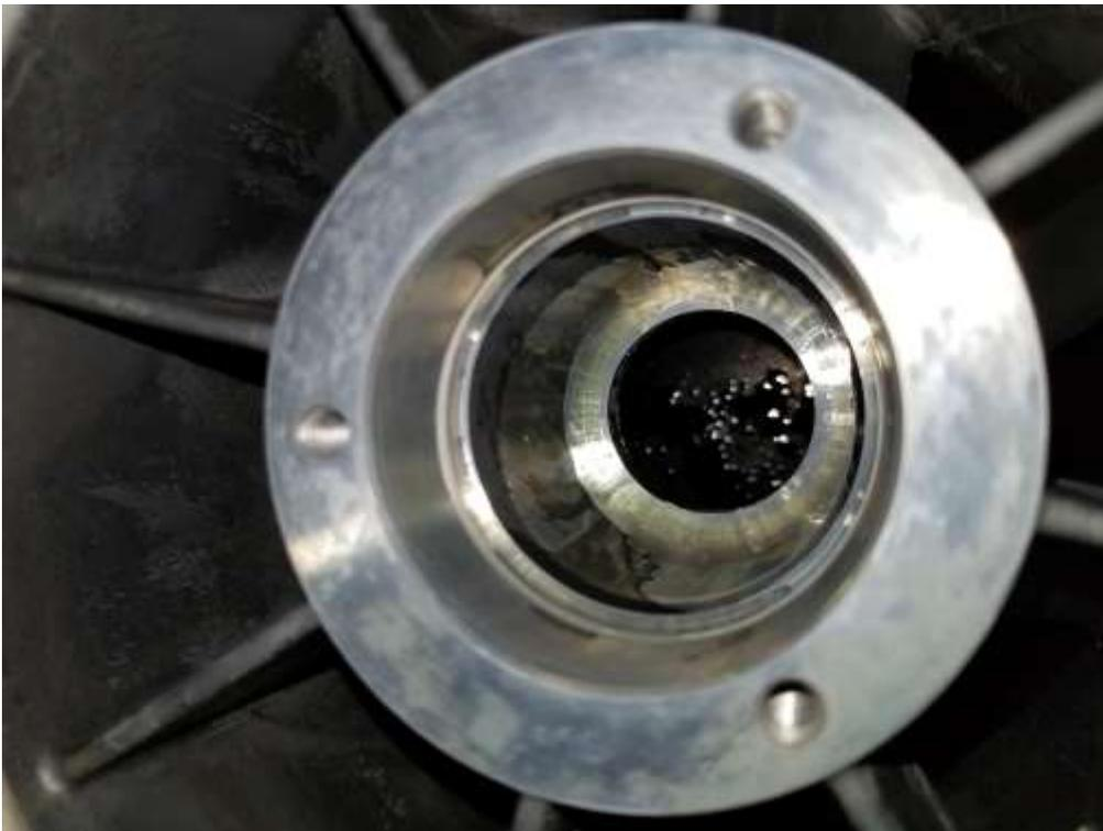
10) Lubricate first main pump bearing.
