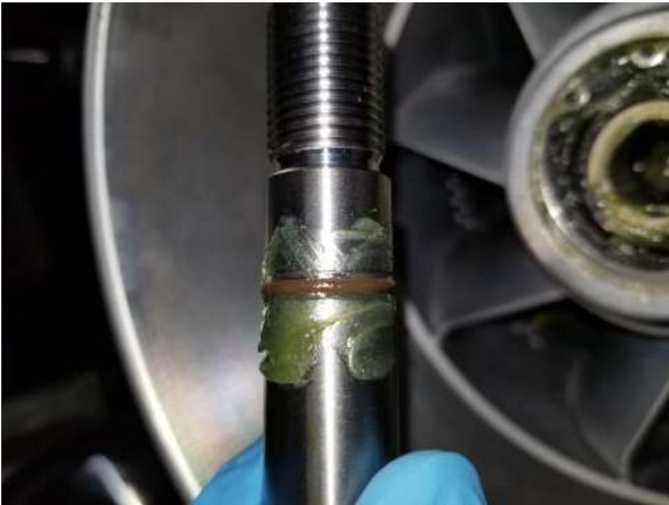
22) Flip pump over, install impeller shaft.
