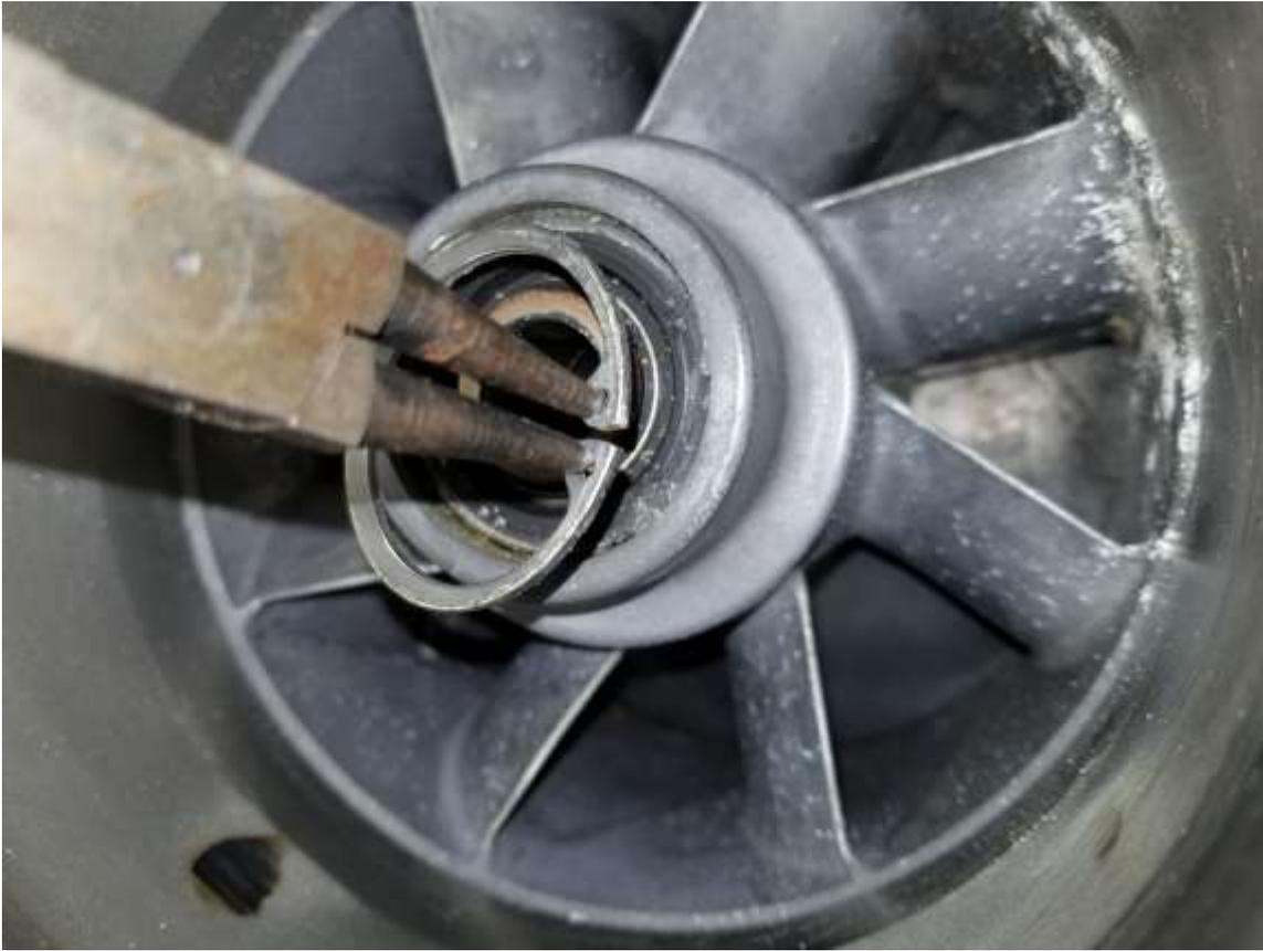
5) Using a rigid screw driver, pry the old seals out from the inner lip. **DO NOT PRY ON THE OUTER SURFACE!**
